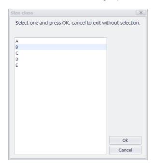
Choose the necessary Stream as active and press **Fill Gangue**. A window for the selection of size class will appear. Choose the necessary size class from the list and press **OK**. You will see a choice of mineral group window. Choose a mineral group and press **OK**. After that, the **Min Particles Size** window will appear. In this window you should enter a minimum particle size and press **OK**.
